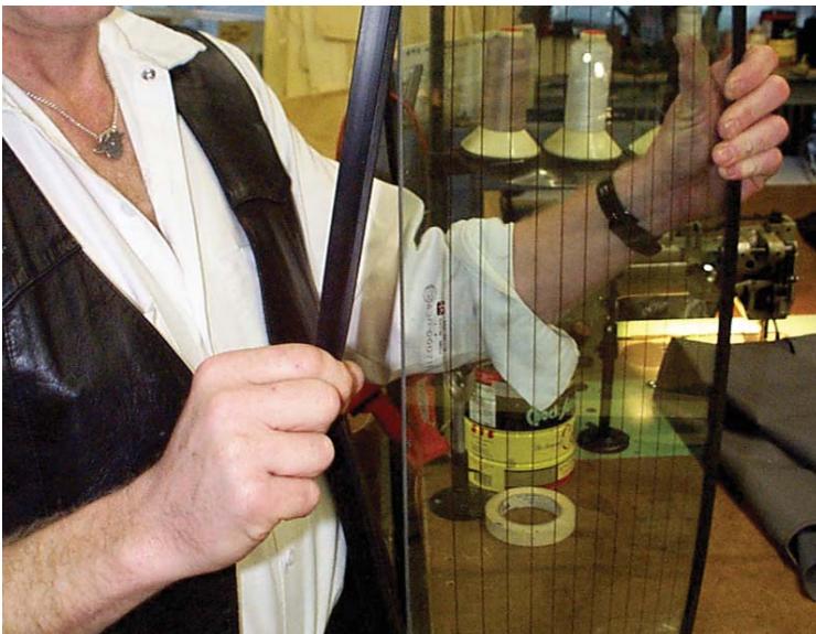
Figure # 3 Stretch the rubber gasket around the glass keeping the wider lip of the gasket on the outside.
