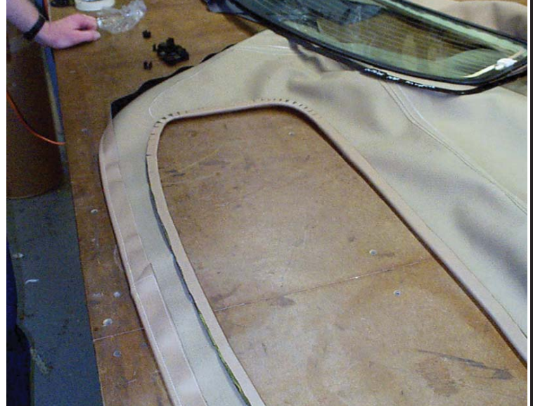
Figure # 2 Apply cement to the inside surface of the metal frame. Fold over window opening and press onto cemented frame, make sure the edge of material is even with the outside of the metal frame. Special Note: Stretch to the corners of the frame first.
