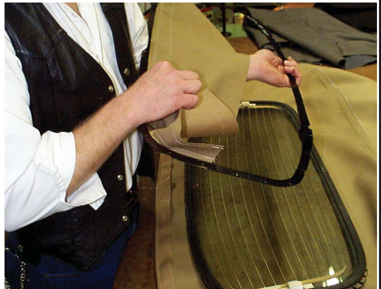
Figure # 4 Place glass with gasket face down on the inside of the frame. Cement upper glass support, to the inside of the metal frame. (New material is supplied or reuse the old one.)
