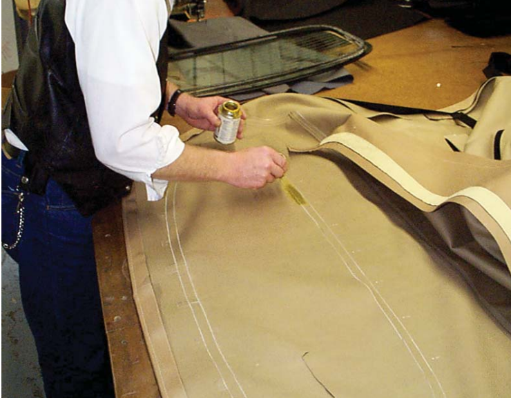
Figure # 1 Apply contact cement between the lines drawn on the lining side of the top around the window opening.
