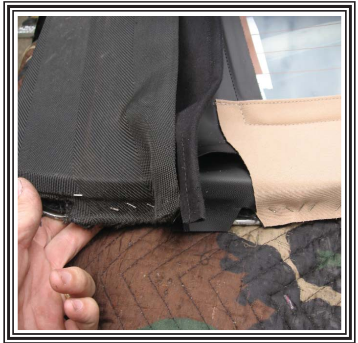
Staple the rear quarter pads to the trim stick.
