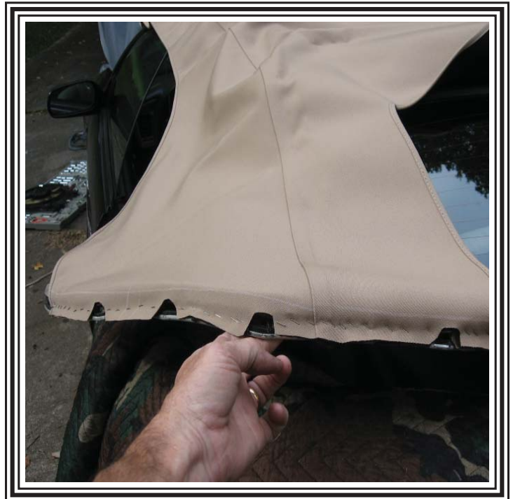
Staple the rear quarters starting at the front of the quarter putting the line at the upper edge of the trim stick and working your way around towards the window.
