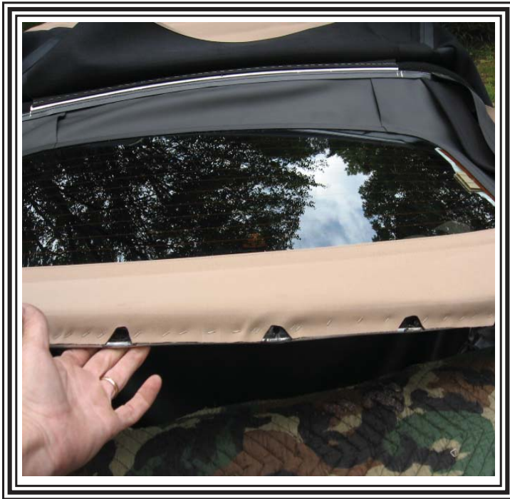
Staple the bottom of the rear window putting the line at the upper edge of the trim stick.
