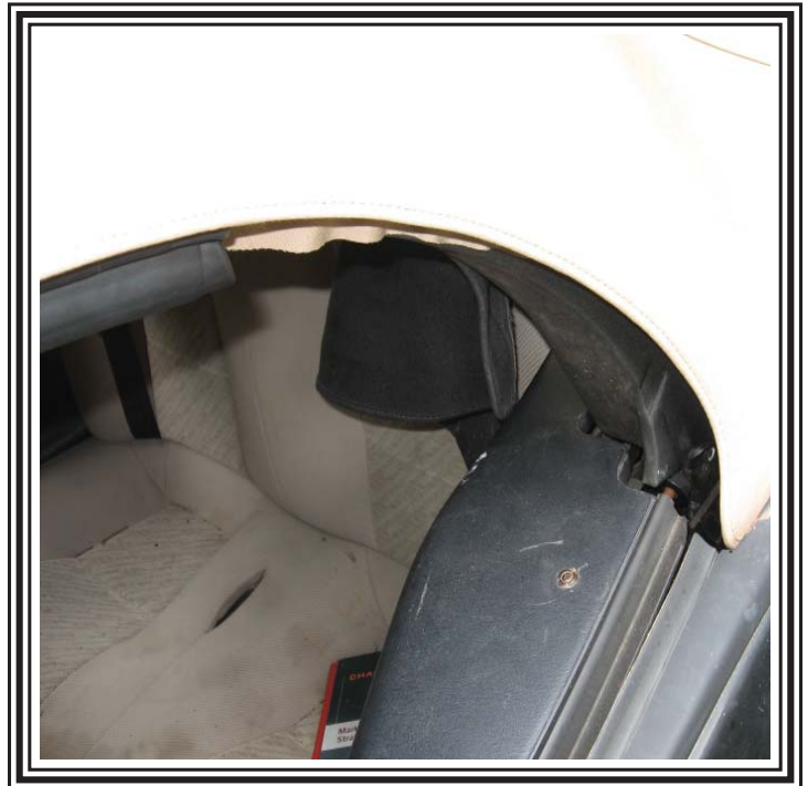
Put back on the channel rubbers.
