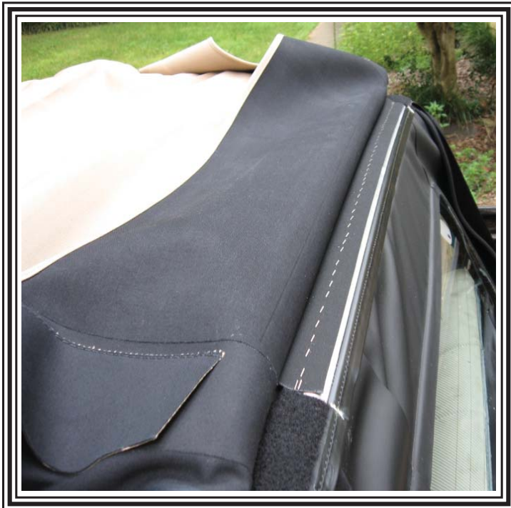
Staple the rear bow listing making sure that the top is centered on the rear bow.
